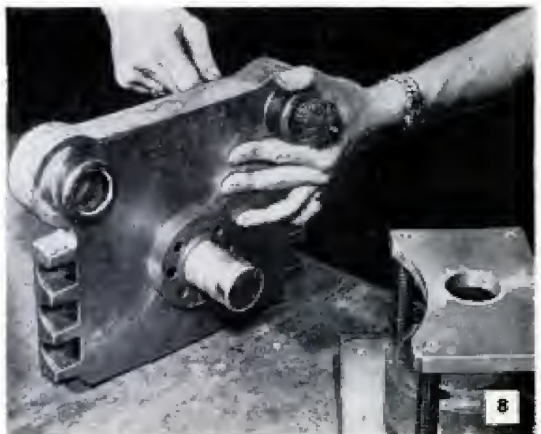
8. ROUND STIFF-BRISTLE BRUSH is especially made for cleaning leader-pin holes in die sets. Bristles are of selected genuine horsehair which is resistant to acids and alkalis common to most detergents and industrial cleaning fluids. It is available in sizes ranging from \frac{3}{8} to 2 \frac{3}{4} -in.-bristle dia.
